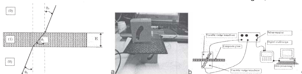
Fig. 2. a) Ultrasonic waves propagation scheme through composite plate, b) US measuring device, gripping mode of the traducers, mounting plate composite between angular transducers and c) principle sketch
