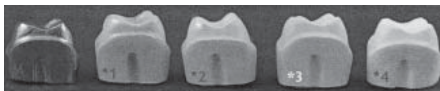
Fig.1. Co-Cr dies coated with spray A (M-control specimen, *n- number of consecutive layers of spray)
